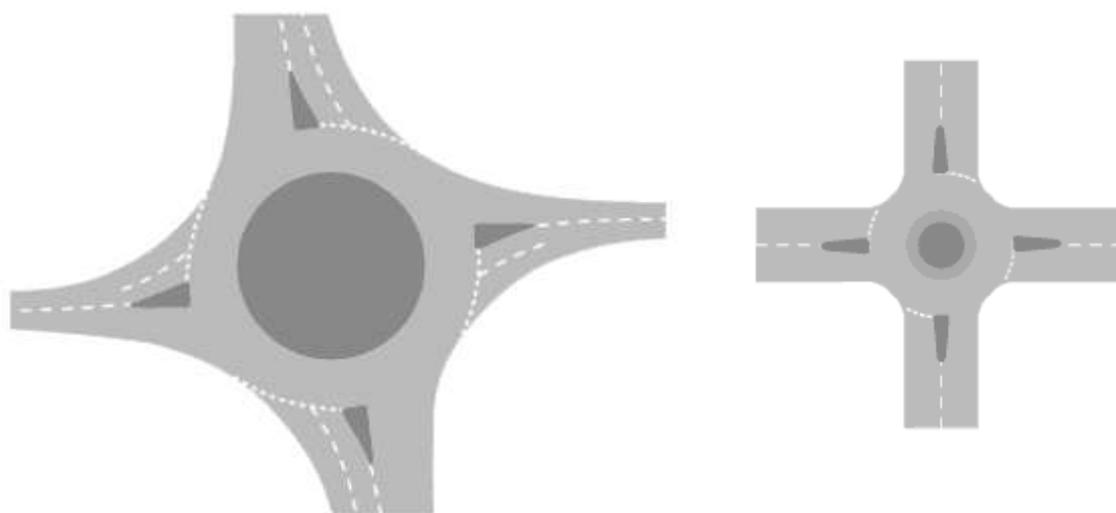
**Figure 1: Comparison of UK Standard (left) and Continental (right) roundabout geometries**
