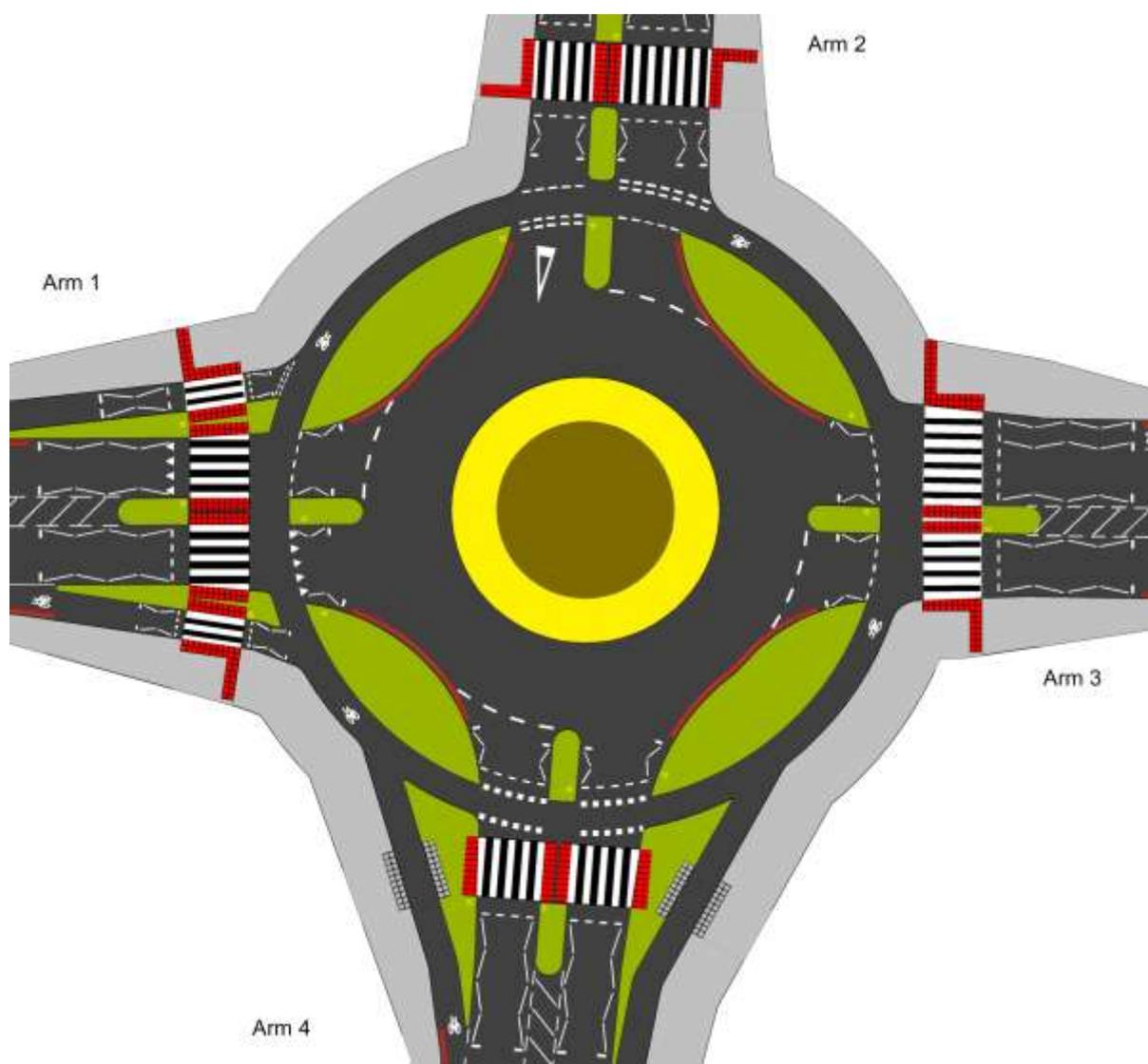
**Figure 4: Layout of the Dutch style roundabout with UK markings**
