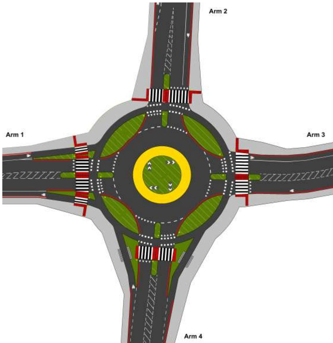
**Figure 2: Layout of the Dutch-style Roundabout with Dutch road markings**
