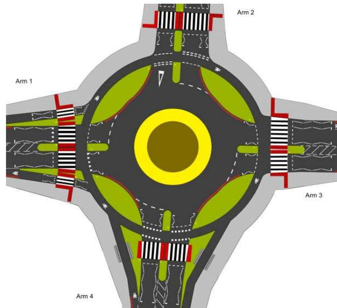
The segregated cycle track is used to keep cyclists away from circulating vehicular traffic. While this forms part of the system of segregated cycle tracks commonly used in the Netherlands, it is also used at roundabouts in urban environments where cyclists typically share roads with other traffic.
