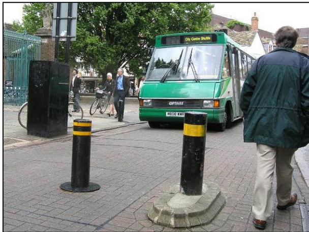
Rising bollards used to admit public transport whilst restricting other vehicular access, Cambridge (note cycle slip being used by pedestrian).
