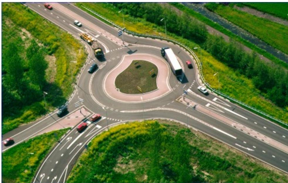
Figure 1. *Turbo-roundabout.*
